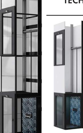
Screw-driven cabin lifts are powered by the rotation of a nut on a screw, and come with their own shaft. Thanks to their driving principle and design, screw-driven cabin lifts do not require a pit, machine room or shaft. These features make them ideally suited for the home.
